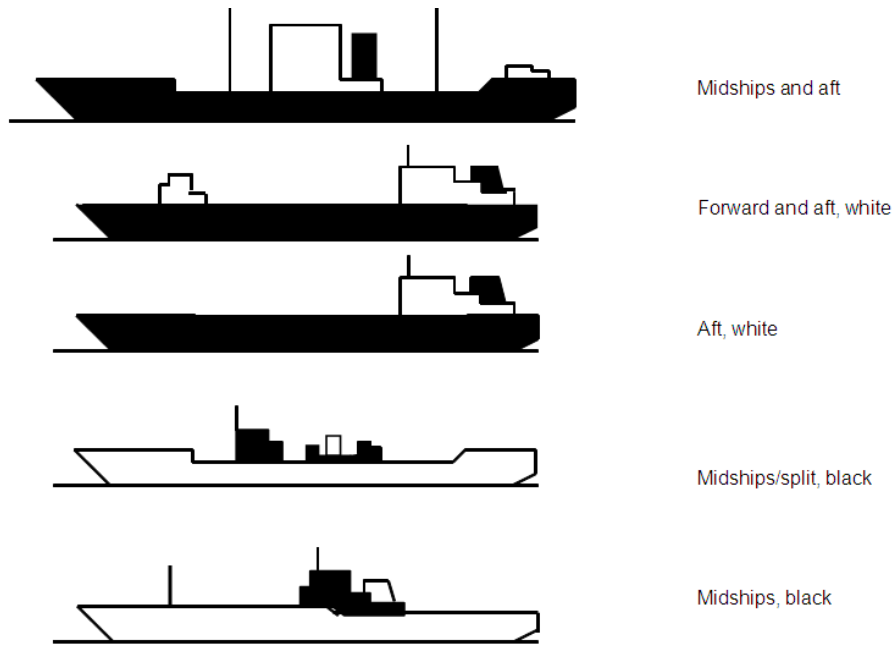
Figure F.1 Superstructure Locations/Colour
